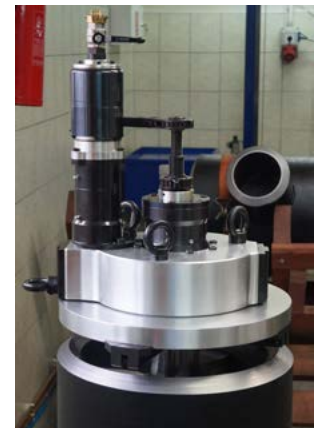
Machining pipe 18" schedule 160
