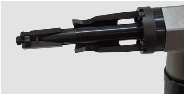
Cutter head design to remove both left and right hand Fins
