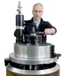
ID Clamping End Prep Tool 7" I.D. to 23,6" O.D. 180 mm I.D. to 600 mm O.D.
