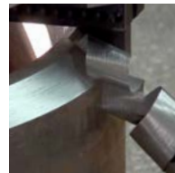
Machining pipe 24" schedule 160
