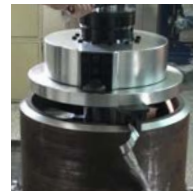
Machining pipe 24" schedule 160
