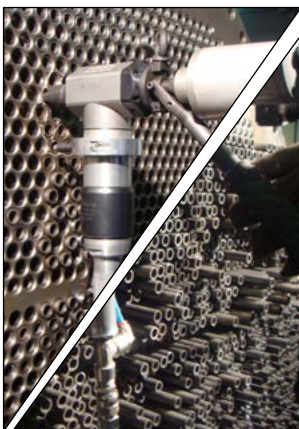
A real application: shortening a bundle. MiniMill can deal with this task quickly and efficiently.
