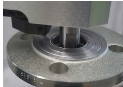
Refaced and re grooved flange with MFM
