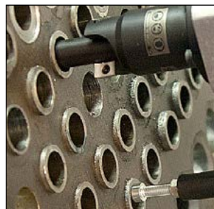
Double sided inserts and fixed diameter heads ensure unsurpassed efficiency and quality. Mechanical stops ensure identical tube projection.
